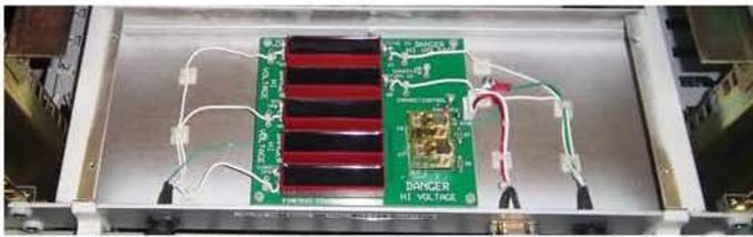
*Close-Up FineTest HV Relay Unit for Hipot*
