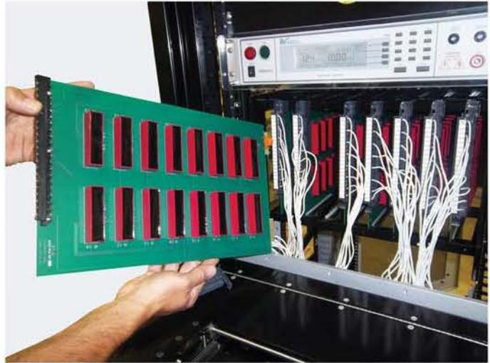
*Close-Up of Dual 8x1 HV Mux Card*
