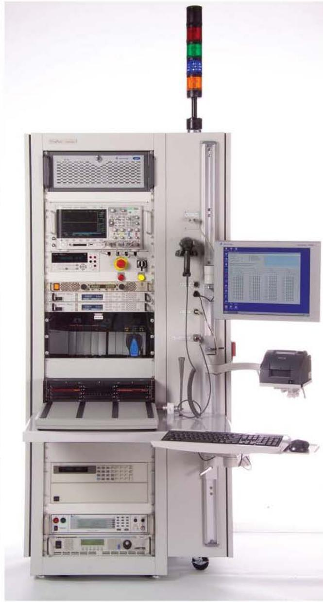
Front view of Tester with Integrated HIPOT
